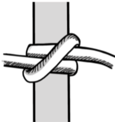
Clove without safety (incomplete)
